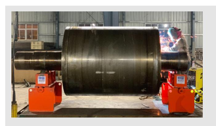
Various pulleys such as key-way, turbine and T-Bottom are produced using automated welding machines to ensure consistency in quality and avoiding human intervention.
